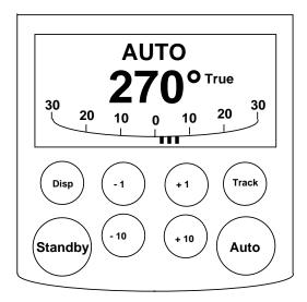
level of response. The higher the response level, the more frequently adjustments will be made by the autopilot. Lower the response level when sailing in large swells.
